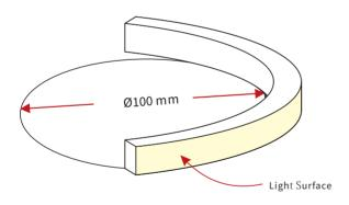
$The\ light can only\ be\ bent\ along\ the\ light\ surface.\ Do\ not\ bend\ smaller\ than\ allowed\ minimum\ bend\ diameter.$
