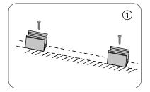
1. Installation of clip Fix the clips and aluminum profile via the screws
