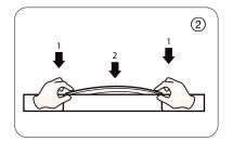
2. Installation Simultaneously install the neon from both ends
