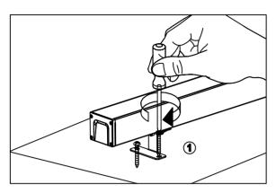
1. Fix the fixture with screws on the surface of the mounted object, make sure the fixing possion.
