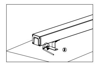
2. Rotate the fixture boy to a suitable projection angle.
