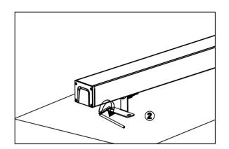
2.Rotate the fixture body to a suitable projection angle.
