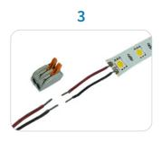
Check the Polarity and connect with locally available connectors
