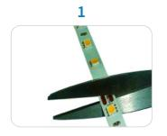
Handle strip carefully. Cut strip on on dotted mark with sharp scissors
