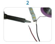
Carefully solder with prepared cables on the marked contacts. Minimise contact with heat tip to avoid heating the PCB
